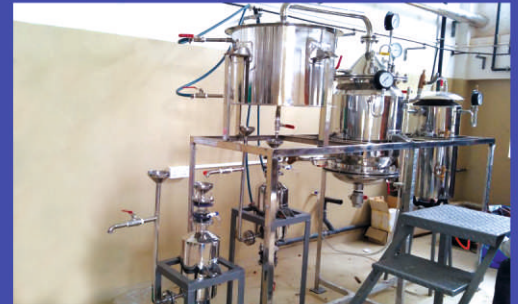
Pilot Scale Distillation Plant
